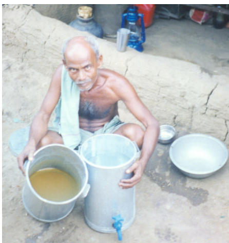
Fig.2: Terafil water filter in GI container used in super cyclone affected areas of Orissa
